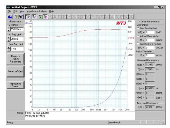
Here is a typical result when measuring a 1.0 mH inductor:
